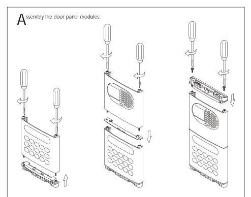
Insert the header DOWN marked in the lower module and fix it by screwing the module shafts.
