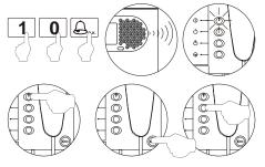
Enter the code of the monitor to be programmed and press the bell key. At this moment the panel will reproduce a sound and the monitor led will blink.
