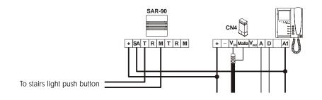
The use of a TF-104 transformer will be necessary to activate a second lock release. IMPORTANT: the lock release must be 12Vc.a. type.
