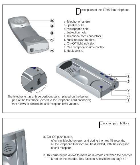
c. If the handset is on the craddle sends a panic call to the porter's exchanges that have enabled the reception of this type of call. If not, allows to call to the master porter's exchange. During call reception and communication progresses allows the lock release activation.
