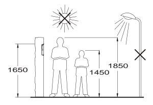
The upper part of the module should be placed at 1,65m. height roughly. The hole dimensions are: 125(W) x 257(H) x 57(D) mm.
