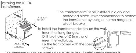
The transformer can be installed on a DIN guide (3 units) simply pressing it. To disassemble the transformer from the DIN guide, use a plain screwdriver to lever the flange as shown on the picture.
