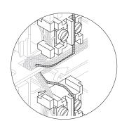
IMPORTANT: link the push buttons common terminal of all the modules. The common terminal of the push buttons contained in a module are linked from factory.
