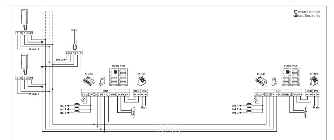
The lock release can be activated at any moment by using an external push button, that must be connected between '~1' y 'CV' terning of the sound module. This function will allows to exit from the building being not necessary the use of a key.
