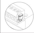
EL551 sound modules for systems with several access doors have a jumper placed on the right side of the terminal connector. This jumper allows to select between two different call types, allowing the user to distinguish which door panel is calling.
