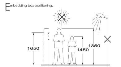
The upper part of the door panel should be placed at 1,65m. height roughly. The hole dimensions will depend on the number of door panel modules.
