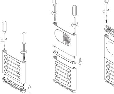
Insert the header DOWN marked in the lower module and fix it by screwing the module shafts.
