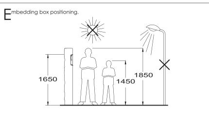
The upper part of the door panel should be placed at 1,65m. height roughly. The hole dimensions will depend on the number of door panel modules.
