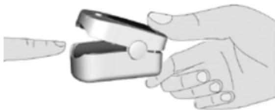
Figure 4 Put Finger into the Sensor
