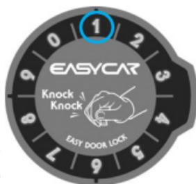
In case that the incorrect passwords are inputted more than 5 times, Easy Door Lock will not be functional for 20 minutes.
