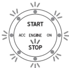
Once you release the parking brake (Auto transmission) or emergency brake (manual transmission) to drive, the red colored light is off.
