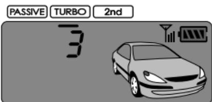
for a selected time of 30 seconds or 2 minutes (you can change the setting in Option menu). This is very useful for turbo charged vehicles to cool down the mechanical components after driving.
