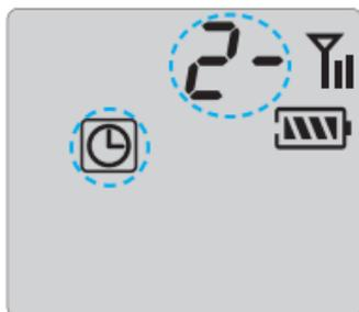
Press the button (🔑+🚗) for 2 seconds and release and then press 🔑 for 2 seconds. Then 🕒 icon appears on the screen. From then on, the vehicle start automatically at reserved time in every 24 hours.
