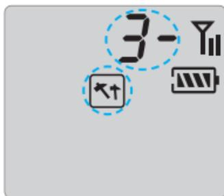
Press button (🔑+🚗) simultaneously for 2 seconds and release, and then continuously press the button 🚗 for 2 seconds to deactivate the shock sensor.
