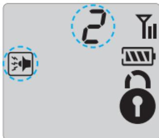
Press button (🔑+🚗) simultaneously for 2 seconds and then press button 🔑 for 0.5 second. to enter this mode, and then all the Icons displayed on LCD disappear and the siren does not operate. The siren, however, operates in
