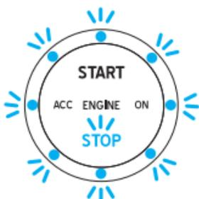
While pressing the foot brake on, press start button for 1 second. Also, the parking brake (Auto transmission) or the emergency brake (manual transmission) should be on at this stage. You will see the engine get started and on the button, it has the red colored light on (Stop).
