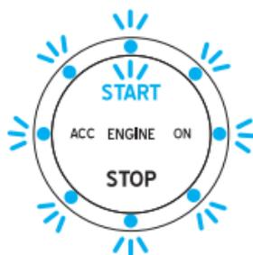
① While pressing the foot brake on, press start button for 1 second. Also, the parking brake (Auto transmission) or the emergency brake (manual transmission) should be on at this stage. you will see the engine is off and the button gets the light on (Start).
