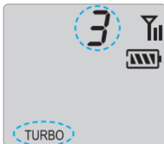
Press (👉+👈) for 2 seconds and release, then press the button 👈 for 0.5 second and release. In this mode, engine continues to run for a selected time of 30 seconds or 2 minutes (you can change the setting in option menu).
