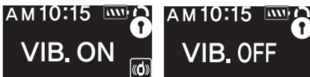
Press button IV for 2 seconds (Vibration on), and press button IV for 2 seconds again to turn it off.
