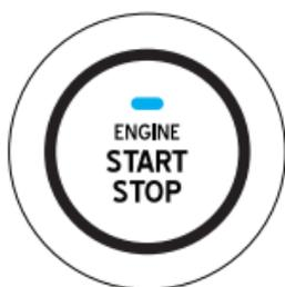
While pressing the foot brake on, press start button for 1 second. Also, the parking brake (Auto transmission) or the emergency brake (manual transmission) should be on at this stage. You will see the engine get started and on the button, it has the blue colored
