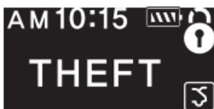
The siren in your vehicle operates even in silent siren mode and chirps for 30 seconds .
