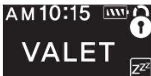
Press button (I+III) simultaneously for 0.5 second to enter this mode.
