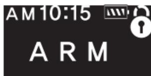
You can lock and arm your vehicle by pressing button I for 0.5 second. The siren chirps and the parking lights flash once each. Also, the sidemirror is being folded.(Optional installation)
