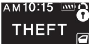
The system recognizes any theft, and activates alarm when doors open by force or with the key while the vehicle is armed.
