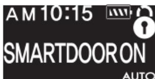
Press button II+III for 2 seconds, then **AUTO** icon appears on the LCD. To cancel it, press II+III for 2 seconds once again. The doors are unlocked when the car owner
