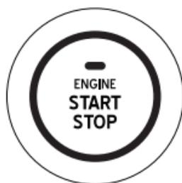
① While pressing the foot brake on, press start button for 1 second. Also, the parking brake (Auto transmission) or the emergency brake (manual transmission) should be on at this stage. you will see the engine is off and the blue Colored Light is off.
