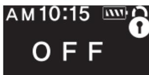
When the vehicle starts,
