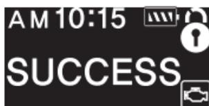
Press and hold button II, for 2 seconds, the remote chirps and the parking lights flash once each. If it fails, the system automatically repeats remote start a maximum of 3 times.
