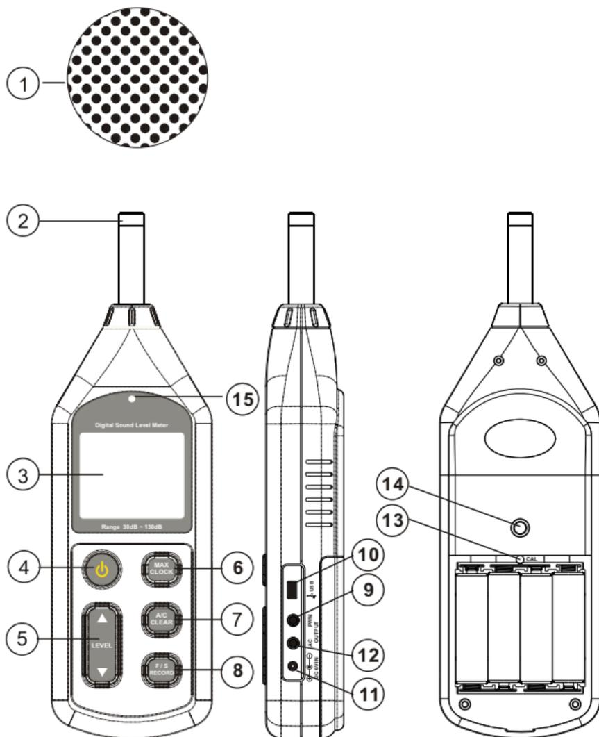
1. Sponge ball (when outdoor use please put on, prevent wind blowing noise disturbing the unit reading)
