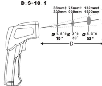
3. Field of view: Make sure the target is larger than the unit's spot size. The smaller the target the close measure distance. When accuracy is critical, make sure the target is at least twice as large as the spot size.
