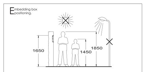
The upper part of the door panel should be placed at 1,65m. height roughly. The hole dimensions are:
