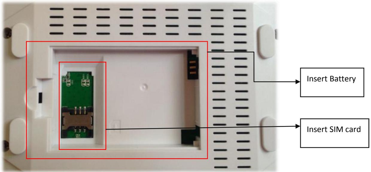
The SIM card and battery interface is positioned at the bottom of this router, and the SIM card slot is under the battery slot.
