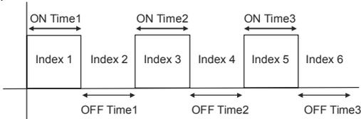
Where ON1 and OFF1 time is for Cadence1 and ON2 and OFF2 is for Cadence2.
