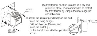
The transformer can be installed on a DIN guide (3 units) simply pressing it.
