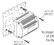
The power supply must be installed in a dry and protected place. It's recommended to protect the power supply by using a thermo-magnetic circuit breaker and to use a ground connection.
