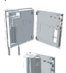
Place the monitor at right angles to the connector and align the attaching holes of the monitor with the attachment hooks of the connector, as it is shown on the drawing.
