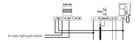
The use of a TF-104 transformer will be necessary to activate a second lock release. IMPORTANT: the lock release must be 12Vc.a. type.
