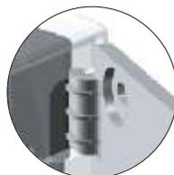
Lock out the monitor. Press the right side till the attachment clip locks the monitor firmly.
