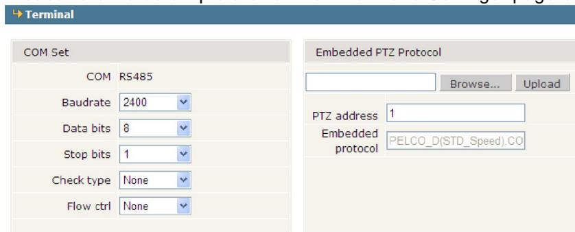
**[Serial port settings]:** When IP camera is connected to RS485 (or RS232) communication or control device (e.g. PTZ decoder, dome camera), the parameters of RS485 (or RS232) need to be set according to the settings of the communication control device (address, protocol, baud rate), and the corresponding protocol need to be downloaded.
