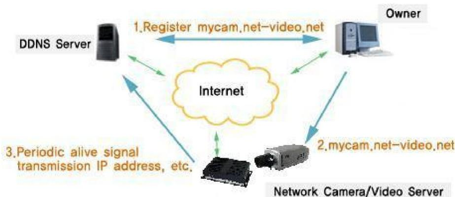
The DDNS process flow diagram of IP camera
