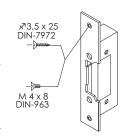
IMPORTANT: the lock release to be used must be 12Vd.c.
