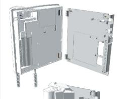
Place the monitor at right angles to the connector and align the attaching holes of the monitor with the attachment hooks of the connector, as it is shown on the drawing.
