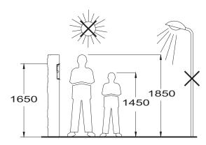
The upper part of the door panel should be placed at 1,65m. height roughly. The hole dimensions are: 131(W) x 131(Al) x 45(D) mm.
