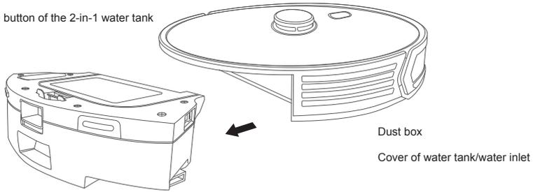
Press the buckle of the dust box to open the dust box.
