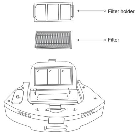
Use a cleaning brush to remove debris from the filter and filter holder. Clean the dust box with running water.
