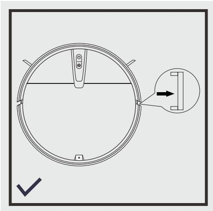
Please remove the white strips on both sides of the bumper before use, otherwise the machine will not work normally
