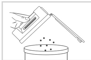
Remove the filter elements. HEPA can be washed with water, and you can tap it to remove dust before washing.
