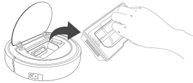
2. Open the dust collector lock and pour the dust and garbage.
