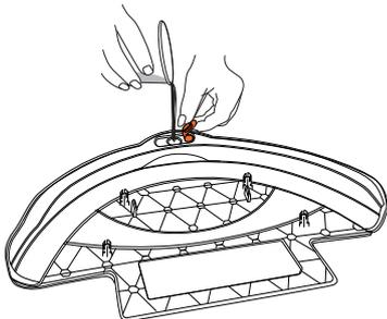
3. Place the bottom of the machine upward, align the positioning column of the water tank with the positioning hole of the carriage at the bottom of the machine, and press the water tank tightly.
