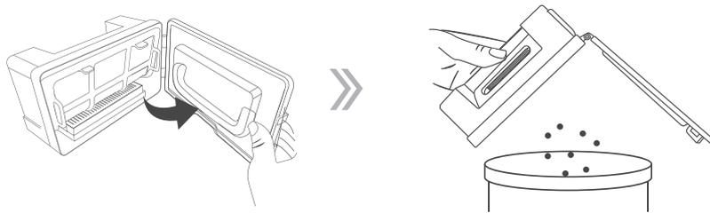
3. Remove the filter elements. HEPA can be washed with water, and you can tap it to remove dust before washing.
