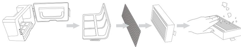
4. Wash the dust collector and the first filter element, dry the dust collector and filter elements, and keep them dry to ensure their service life
