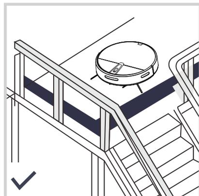
Guardrails shall be placed at the edge of the double layer to ensure the safe operation of the product.
