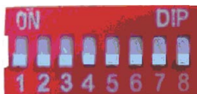
Switch Status when the system expand to 8 C.O.line
